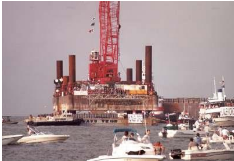
The Karlissa B, the jack-up barge has raised the Hunley and will lower her onto the barge. The barge on the right was used as a breakwater.
