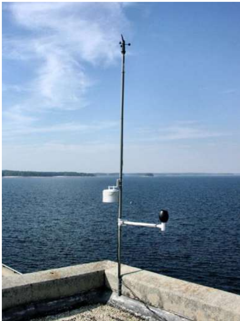
Wind, temperature and rainfall sensors mounted atop the J. Strom Thurmond Reservoir along the Georgia/South Carolina state line.
